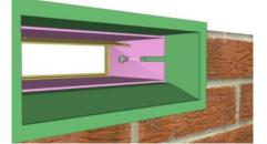
From the back, run a bead of clear silicon along the joint of the front and rear sections.
